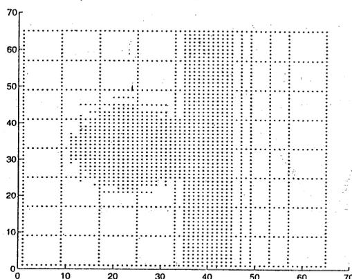
This second example is of a pulse in an isolated region of the domain. The grid selected for this pulse is very dense in the region of the pulse and sparse in the remainder of the domain.
