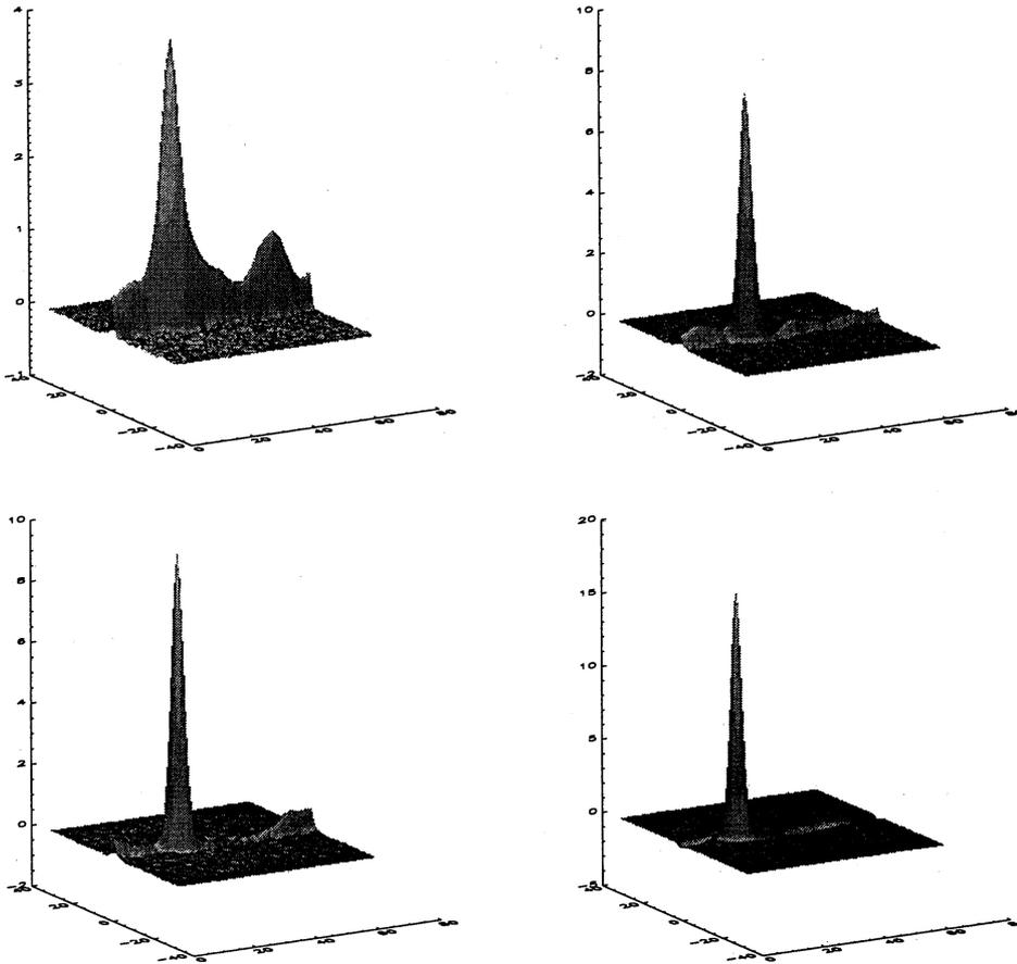
Figure 2: Randomly forced  $-\omega(t)$  field, tube evolution at times: 320 (upper left), 360 (upper right), 400 (lower left), 500 (lower right). The vertical scale (vorticity amplitude) grows with time: fast during roll-up (approximately from 4 to 18 in the frames shown), slowly and fluctuating afterwards. The amplitude of the center line layer decreases.
