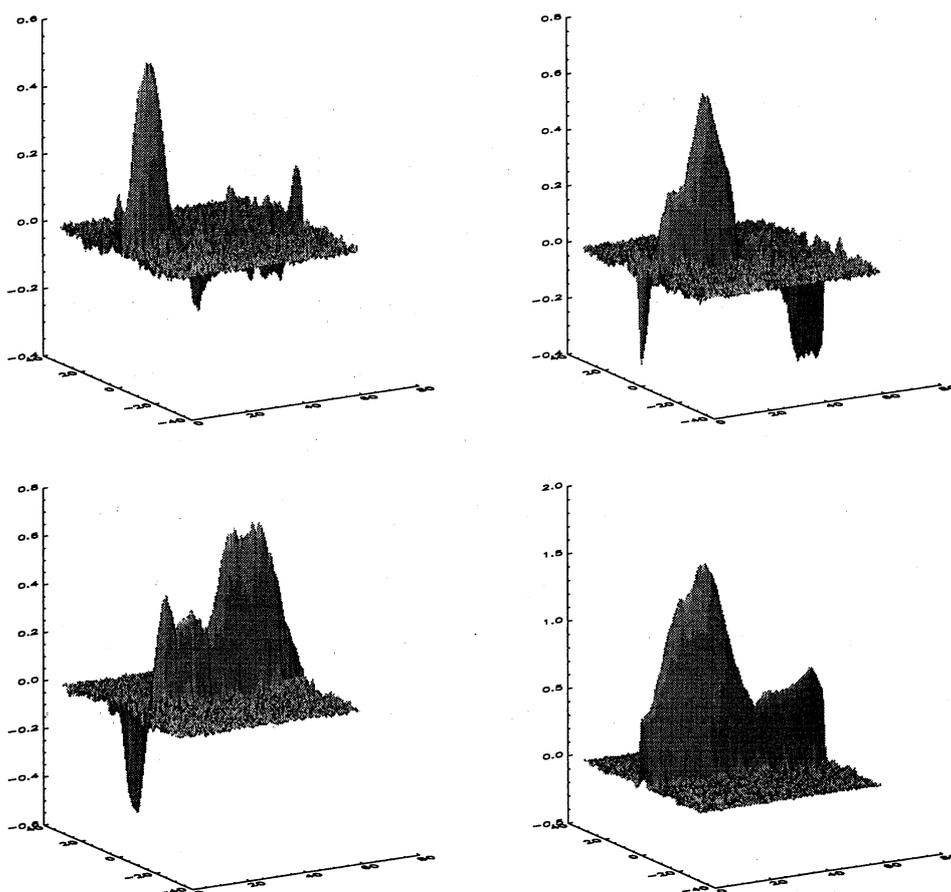
Figure 1: Randomly forced  $-\omega(t)$  field, early times: 10 (upper left), 100 (upper right), 250 (lower left), 270: layer (lower right). The maximum vorticity amplitude at the center line remains about 0.5–0.6, except for the peak in the last frame which has a maximum about 2.0 and shows the initial growth of a tube-like structure.
