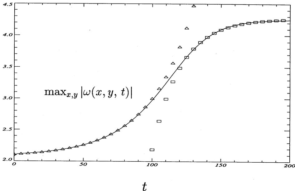
Figure 3: Exponential growth and saturation of the maximum vorticity. Solid line: numerical data of vorticity maxima of perturbed Burgers vortex layer,  $R = 2.6$  and  $L = 16$ . Triangles: growth rate 0.0315, exponential fit. Squares: saturation rate  $-0.049$ , exponential fit.
