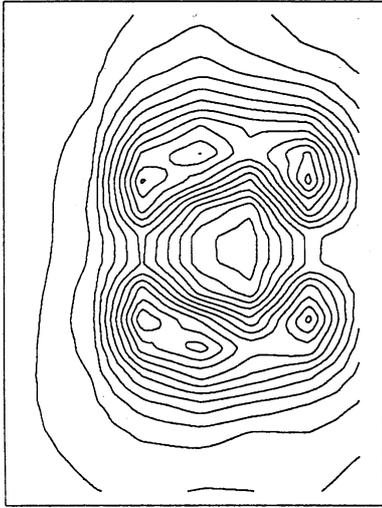
Figure 7: End view of modeled  $P$  at  $t = 350$  in the  $y - z$  plane at  $x = 52.5\theta_0$  from mixing layer; the same portion as in Fig.1 is shown, and  $R_{ij}$  terms implied by the Smagorinsky model ( $0.0 \sim 0.00025(0.00002)$ ).
