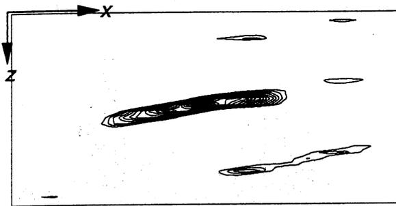
Figure 6: Top view of the conditionally averaged GS normal vorticity  $\overline{\omega}_y$  in the  $x-z$  plane at  $y_+ = 12.0$  from channel flow ( $8 \sim 25(1)$ )
