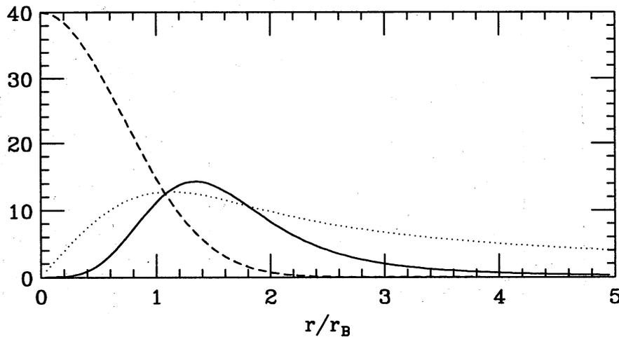
Figure 1: Dashed line, the axial vorticity  $\omega$ ; dotted line, the azimuthal velocity  $v_\theta$ ; solid line, the local energy dissipation rate  $\varepsilon_{\text{loc}}$  of the Burgers' vortex.  $r_B = 1$ ,  $\nu = 0.1$  and  $R_\Gamma \equiv \Gamma/\nu = 1257$ .
