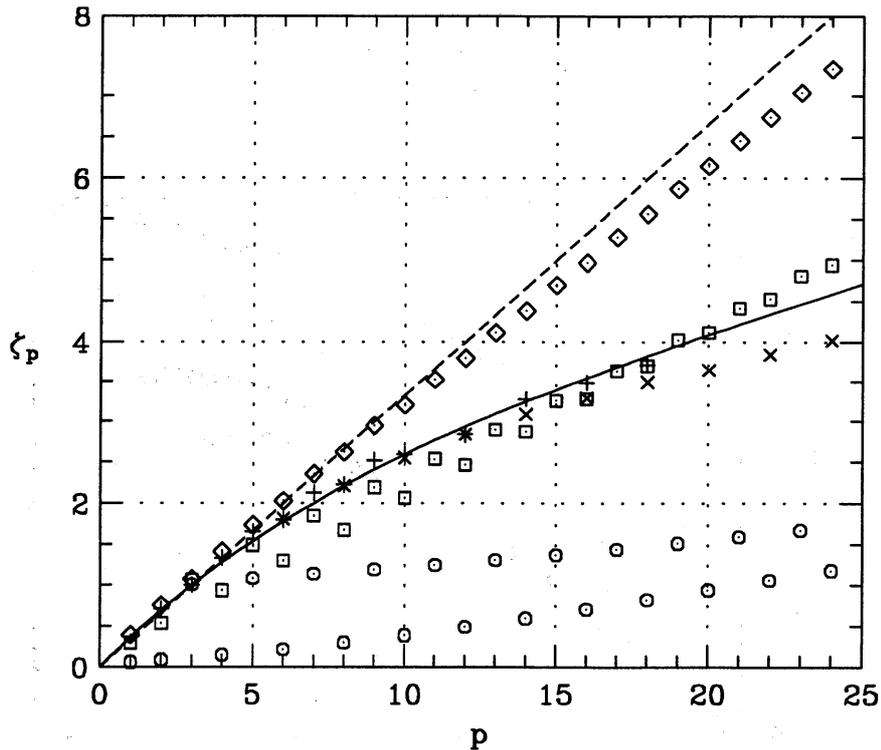
Figure 4: The exponent  $\zeta_p$  of the structure function  $S_p$  shown by  $\diamond$ ,  $\square$  and  $\odot$  which are as in figure 3. dashed line, K41 (1.13); solid line, log-Poisson model (1.17);  $\times$ , DNS at  $R_\lambda = 150$ , Vincent & Meneguzzi (1991) [1];  $+$ , jet at  $R_\lambda = 852$ , Anselmet *et al.* (1984) [11].
