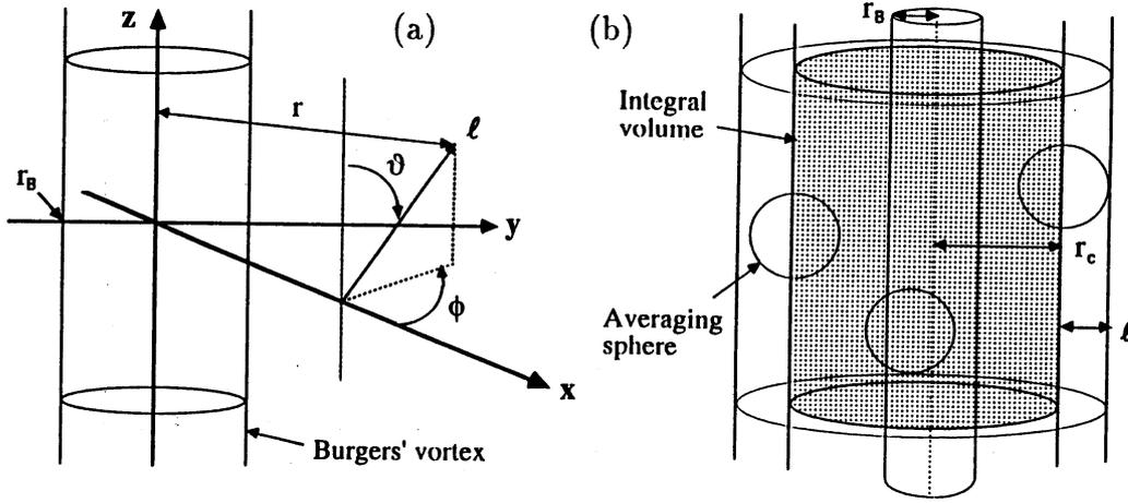
Figure 2: (a) The coordinate system at spherical average with respect to the running point  $\boldsymbol{x} + \boldsymbol{\ell}$  where the reference point  $\boldsymbol{x}$  and the separation length  $\ell$  are fixed. (b) The integral space with respect to the reference point  $\boldsymbol{x}$ .
