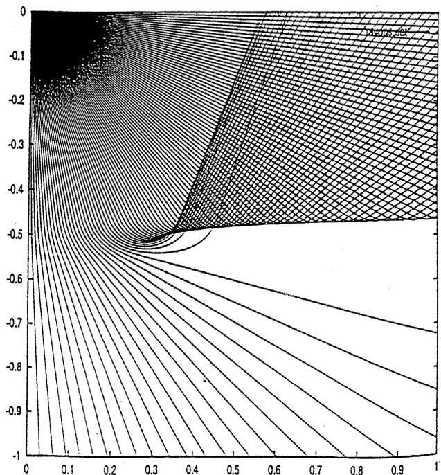
FIG. 9 One hundred rays shot with regularly spaced initial directions.
