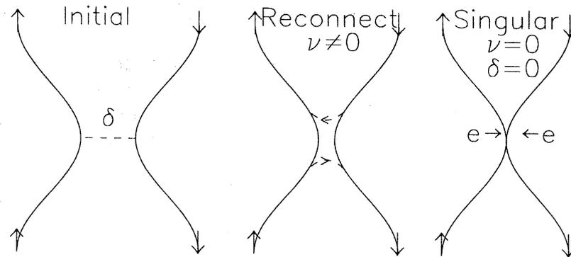
Figure 1: Diagram of the interaction of anti-parallel vortices. From an initial condition of anti-parallel vortices separated at their closest approach by  $\delta$ , if  $\nu \neq 0$  there is reconnection that forms new vortices indicated by the dashed curves. However, if  $\nu = 0$ , a singularity can form when  $\delta = 0$  if the vortices are pushed together by the self-induced strain indicated by  $e$ .
