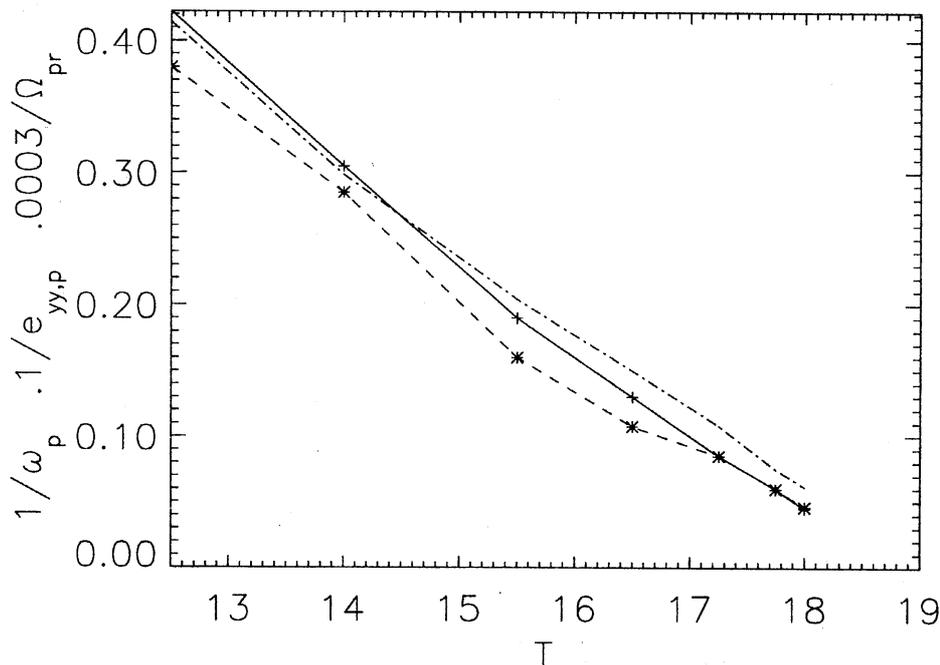
Figure 2: Dependence of  $1/\|\omega\|_\infty$ ,  $1/\|e_{yy}\|_\infty$  and  $1/\int dV \omega_i e_{ij} \omega_j$  on time from the anti-parallel Euler calculation [14] showing convergence to a singular time of about  $T = 18.7$ .
