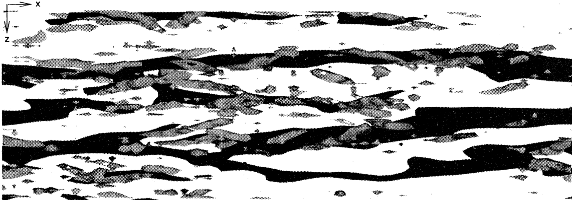
Figure 1. Lifted low-speed streaks (black) illustrated by u' < 0 at y^+ = 20 and streamwise vortices (grey) indicated by the Jeong & Hussain (1995) vortex definition in the region 0 < y^+ < 60 .
