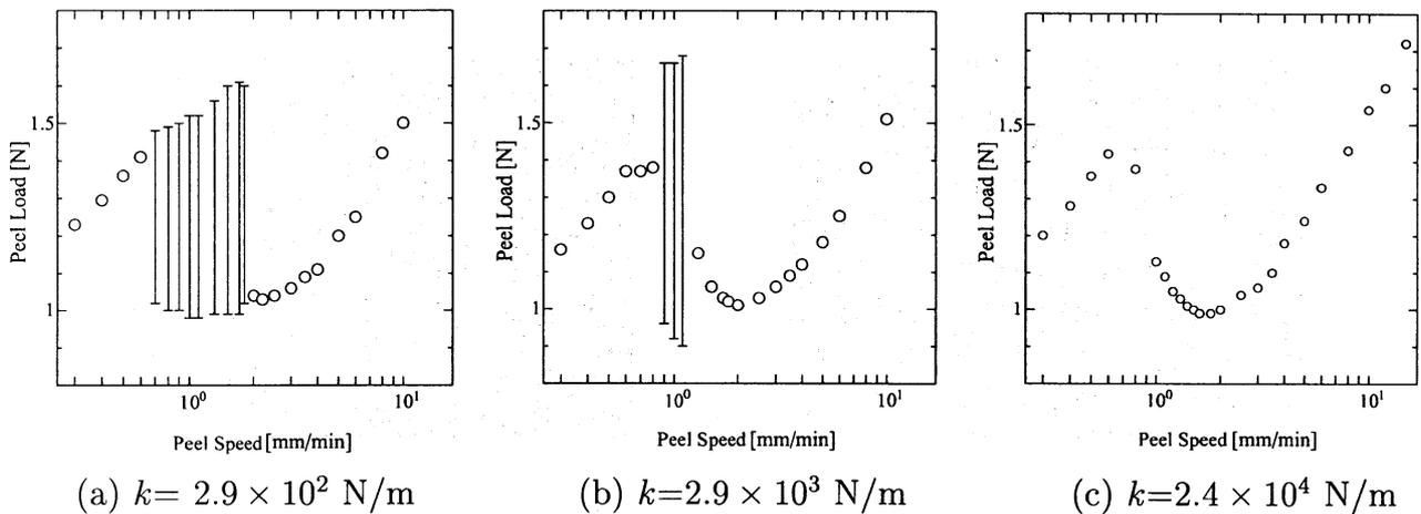
Figure 2: Peel load as a function of peel speed  $V$  in three cases with a different spring constant. (a)  $k = 2.9 \times 10^2$  N/m, (b)  $k = 2.9 \times 10^3$  N/m, (c)  $k = 2.4 \times 10^4$  N/m. The bar represents the amplitude of the oscillatory motion in peel load at each fixed peel speed.
