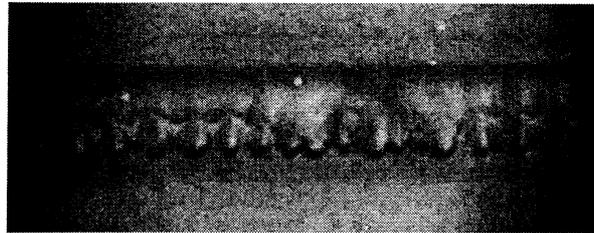
Figure 8: A failure front in the case of a spatio-temporal intermittent pattern. Two kinds of failure morphologies, namely, morphologies in low-speed pattern and high-speed pattern coexist. The actual size of this figure is  $1.9 \text{ mm} \times 0.75 \text{ mm}$ .
