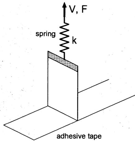
Figure 1: Schematic representation of the experimental setup.
