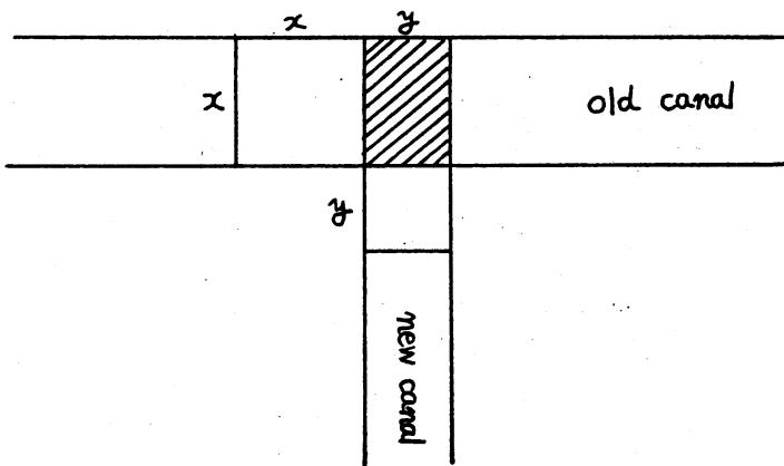
The shadowed area is deeper by 1 kus than the bottom of the canal.
