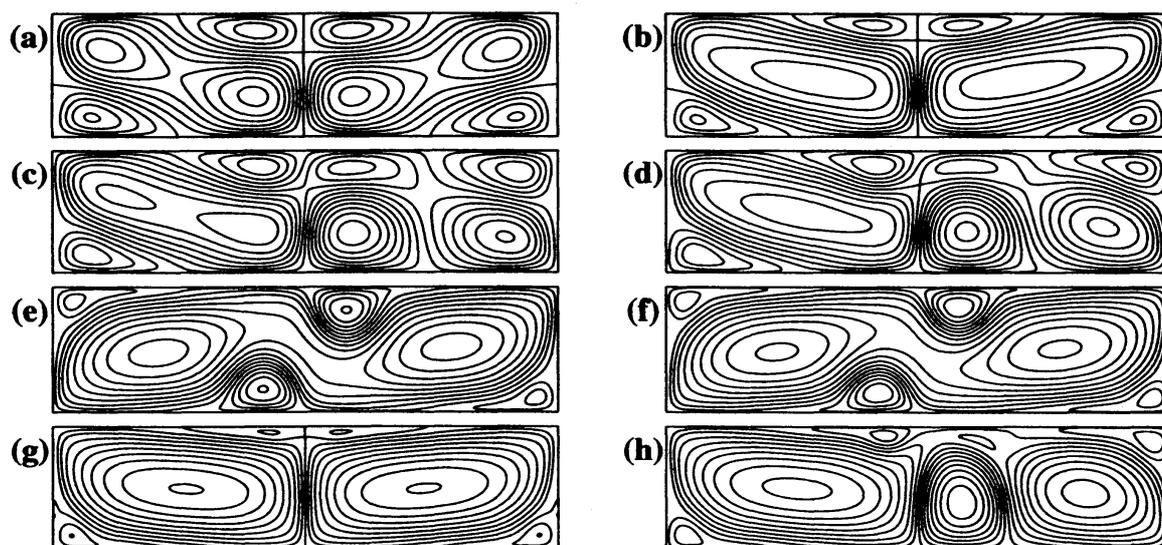
**FIGURE 6.** Streamlines of various steady flows. (a):  $Re = 140$ , (b):  $Re = 230$ , (c):  $Re = 180$ , (d):  $Re = 240$ , (e):  $Re = 700$ , (f):  $Re = 1000$ , (g):  $Re = 1000$ , (h):  $Re = 1000$ .
