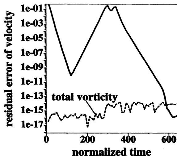
FIGURE 4. Residual error and total vorticity ( $Re = 280$ ).
