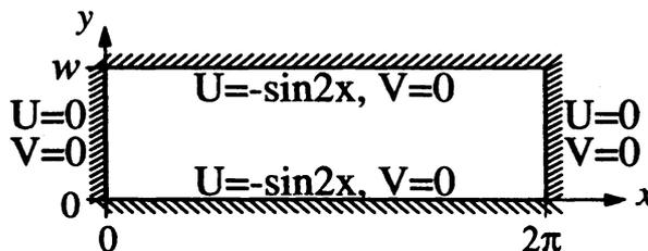
FIGURE 2. The 2D box for simulation.
