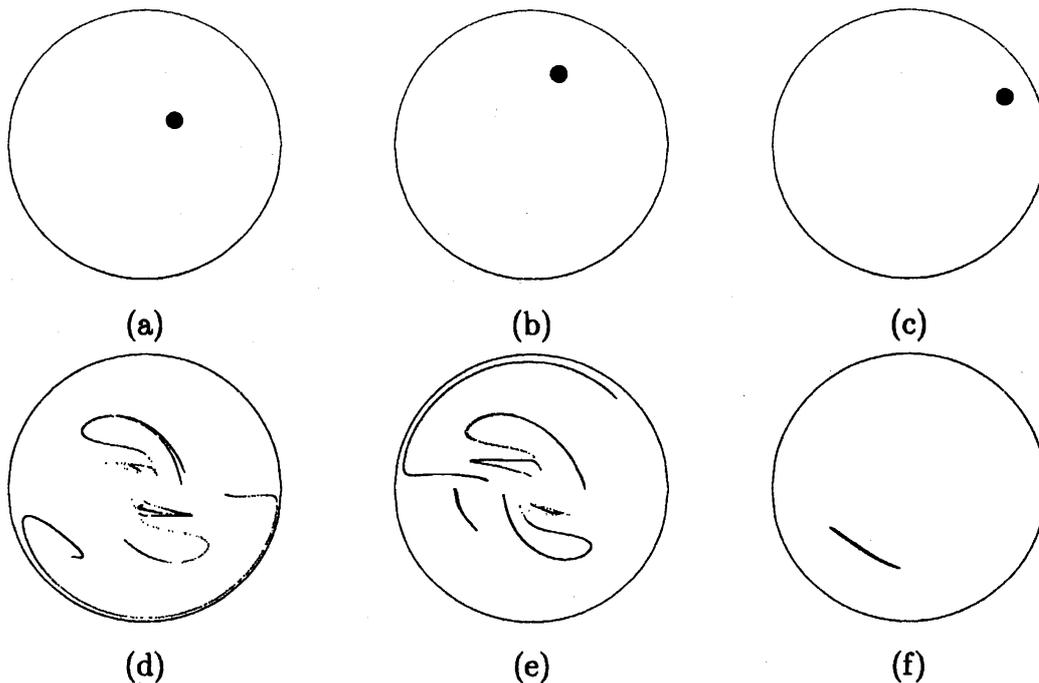
Figure 9: Time evolution of small blobs. Each blob has radius 0.06.  $\alpha = 0.5$ ,  $\beta = 0.03$ , and  $a = 1.0$ . Blobs in (a) and (b) which are close to the lines of separation and that in (c) which is not close to the lines evolve to (d), (e) and (f), respectively.
