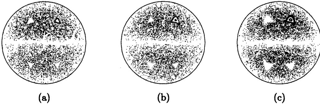
Figure 5: Poincaré sections based on  $M_{I_1/2}$ .  $\alpha = 0.5$  and  $\beta = 0.01$ . (a)  $a = 1.85$ , (b)  $a = 2.33$ , (c)  $a = 3.0$ . The initial locations of fluid particles and the period of plotting are the same as Fig.4.
