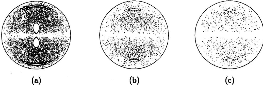
Figure 4: Poincaré sections based on  $M_{I_1/2}$ .  $\alpha = 0.5$  and  $a = 1.0$ . (a)  $\beta = 0.01$ , (b)  $\beta = 0.03$ , (c)  $\beta = 0.1$ . 83 fluid particles are initially placed on square grid points of interval 0.1 in the first quadrant. Their trajectories are calculated up to  $t = 100$ .
