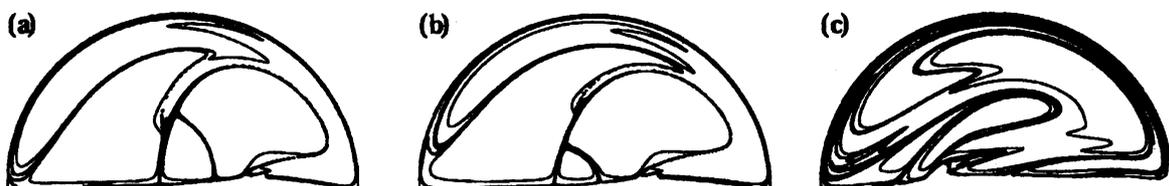
Figure 10: Contours of the residence time based on the 98500 trajectories starting from the initial positions on  $z = l_1/2$ . The initial positions are on square grid points of interval 0.01 on the upper part of the cross-section.  $\alpha = 0.5$ . (a)  $\beta = 0.01$ ,  $a = 1$ , (b)  $\beta = 0.01$ ,  $a = 1.85$ , (c)  $\beta = 0.03$ ,  $a = 1.85$ .
