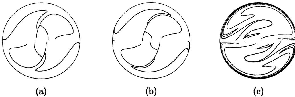
Figure 8: Lines of separation,  $U_{l_1/2}^1$ .  $\alpha = 0.5$ . (a)  $\beta = 0.01$ ,  $a = 1.0$ , (b)  $\beta = 0.01$ ,  $a = 1.85$ , (c)  $\beta = 0.03$ ,  $a = 1.85$ . The initial positions of 40000 trajectories calculated here are uniformly placed on the lines  $10^{-5}$  upstream from the leading edges.
