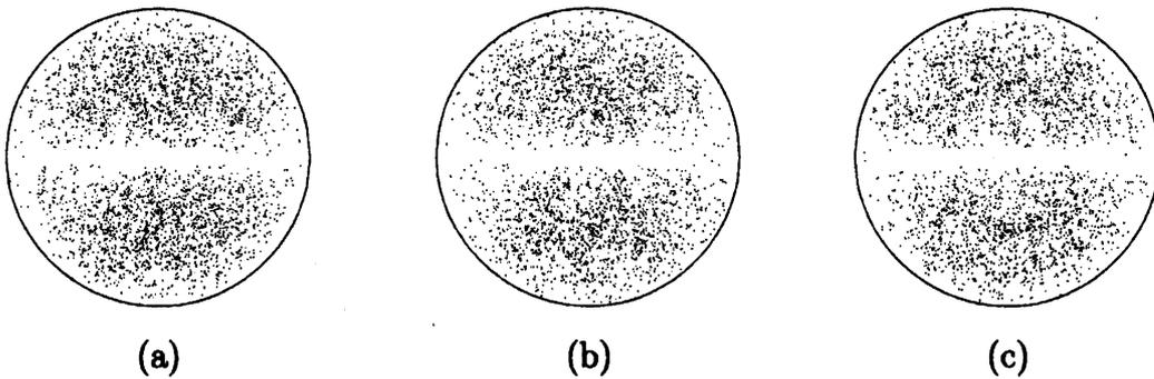
Figure 6: Poincaré sections based on  $M_{I_1/2}$ .  $\alpha = 0.5$  and  $\beta = 0.03$ . (a)  $a = 1.85$ , (b)  $a = 2.33$ , (c)  $a = 3.0$ . The initial locations of fluid particles and the period of plotting are the same as Fig.4.
