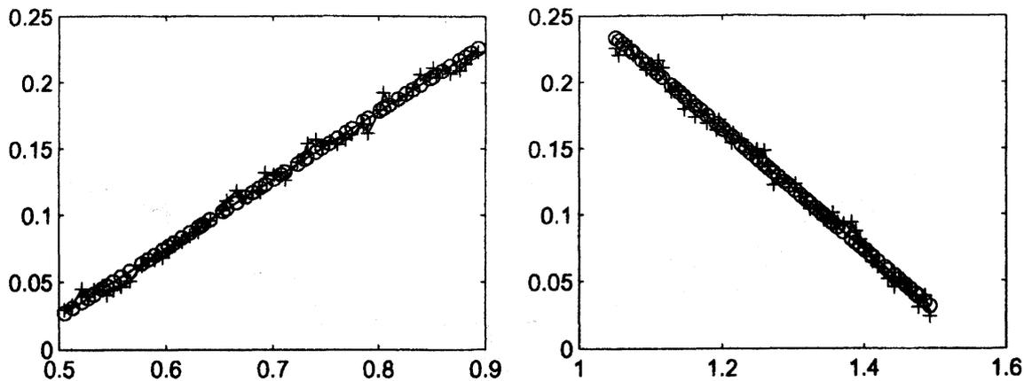
Figure 4: Center of mass for particles on left and right slopes (+) and least squares fit (o) for the determination of the angle of repose.
