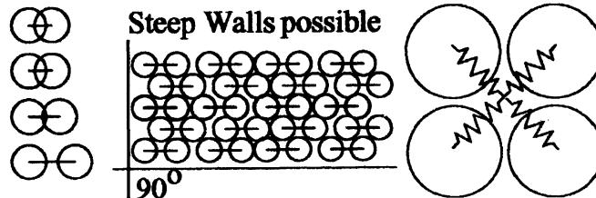
Figure 1: Sketch for the dumbbell-model by Galas (left) for different elongations, resulting in the possibility of a stacking with  $90^\circ$  slope (middle) and clover-leaf-model by Pöschel (right).
