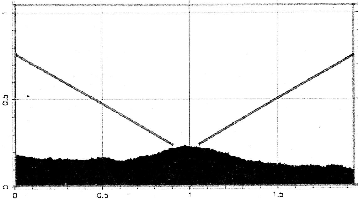
Figure 12: Final configuration for coefficient of friction  $\mu = 0.2$ , particle elongation 1.4 and five corners: Most of the bulk is fluidized, but in the middle below the opening of the hopper, a heap with straight slopes is still recognizable.
