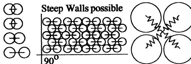
Figure 1: Sketch for the dumbbell-model by Galas (left) for different elongations, resulting in the possibility of a stacking with 90° slope (middle) and clover-leaf-model by Pöschel (right).
