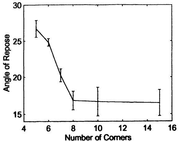
Figure 8: Dependence of the angle of repose on the number of corners of non-elongated nearly regular polygons, averages and error-bars calculated for six slopes /independent configurations,  $\mu = 0.6$ .
