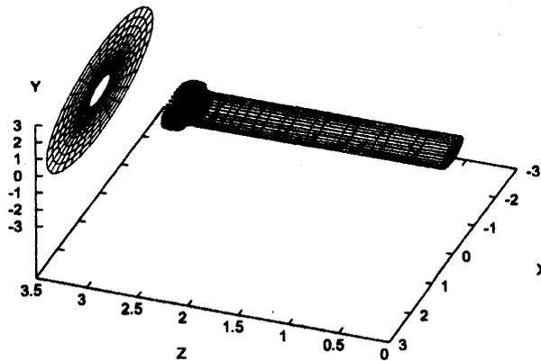
Figure 2: Distribution of bound vortex filament panels on the nozzle and the end plate. The startup vortex of the free jet is also shown in the figure. [In the text the notation  $\mathbf{x} = (x_1, x_2, x_3)$  is used, rather than the notation  $(x, y, z)$  shown in this and in the following figures.]
