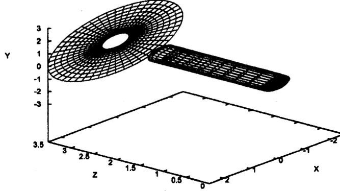
Figure 1: Solid surfaces represented by vortex panels. The mean flow-generating panels are placed at  $z = 0.0$ , the nozzle exit at  $z = 2.5$ , and the end plate at  $z = 3.5$ .
