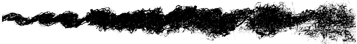
Fig. 4 Distribution of coherent fine scale eddy in spatially-developing turbulent mixing layer
