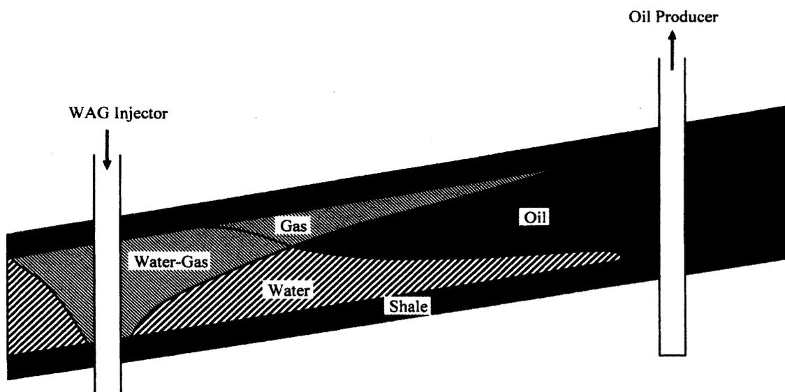
Figure 1: WAG Enhanced Oil Recovery (schematic picture)
