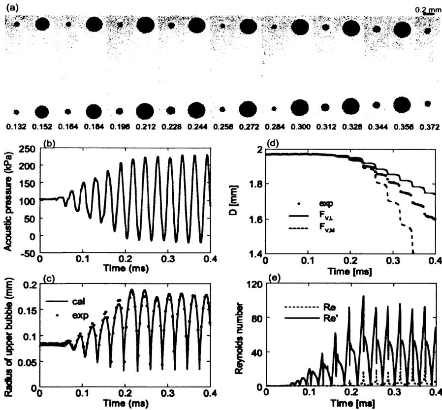
Fig. 3 Attractive motion of a pair of bubbles under strong acoustic forcing. (a) Selected frames of images captured by using high-speed video camera with elapsed time below each image in ms. (b) Liquid pressure measured in experiment and used in the calculation. Evolution of (c) radius of upper bubble, (d) separate distance  $D$  between two bubbles, and (e) actual Reynolds number  $Re$ , and Reynolds number based on the radial motion  $Re'$ .
