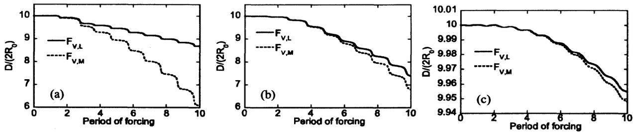
Fig. 5 Time evolution of separate distance between two bubbles obtained by numerical calculation: (a)  $v=50 \text{ mm}^2/\text{s}$ ,  $P_a=130 \text{ kPa}$ , (b)  $v=5 \text{ mm}^2/\text{s}$ ,  $P_a=50 \text{ kPa}$ , (c)  $v=5 \text{ mm}^2/\text{s}$ ,  $P_a=5 \text{ kPa}$ .
