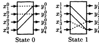
Figure 3: A graphical representation of the 4-RLEM 4-289. Solid and dotted lines describe the input-output relation for each state. A solid line shows the state changes to another, and a dotted line shows the state remains unchanged.
