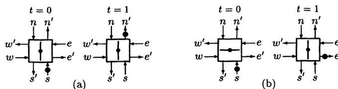
Figure 1: Operations of an RE: (a) the parallel case (state V with input  $s$ ), and (b) the orthogonal case (state H with input  $s$ ).
