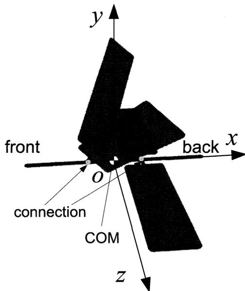
Fig. 2: The 3D flapping wing model and the set of axes fixed to the body ( $o-xyz$ ).
