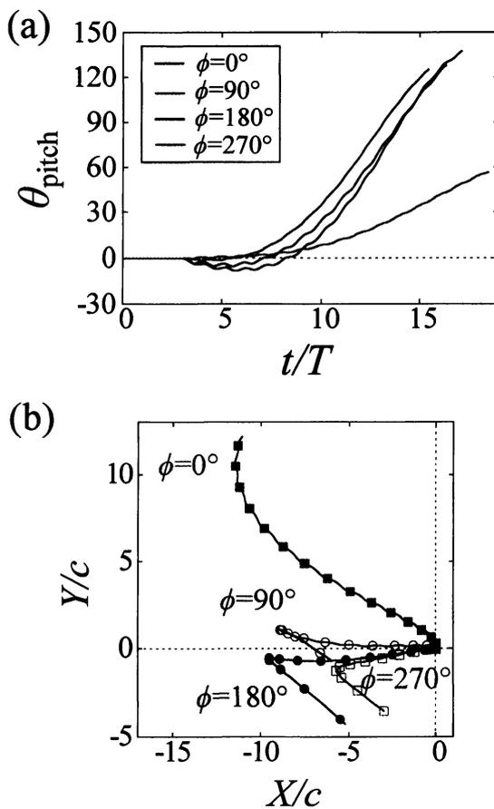
Fig. 13: (a) Time variations of the pitching angle of the body for the 3D flapping wings and (b) the trajectories of the COM for the 3D flapping wings. In (b), the initial position of the COM is  $(X/c, Y/c) = (0, 0)$ , and the dots indicate the position of the COM when the hindwings are at top dead point.
