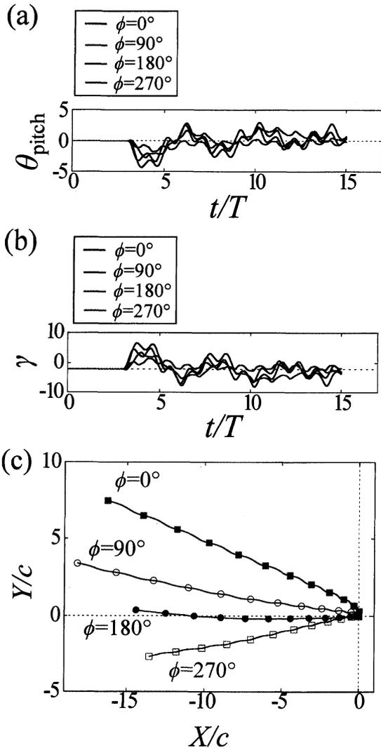
Fig. 15: (a) Time variations of the pitching angle of the body for the 3D flapping wings, (b) time variations of the lead-rag angle of the body for the 3D flapping wings, and (c) the trajectories of the COM for the 3D flapping wings. In (b), the initial position of the COM is  $(X/c, Y/c) = (0, 0)$ , and the dots indicate the position of the COM when the hindwings are at top dead point.
