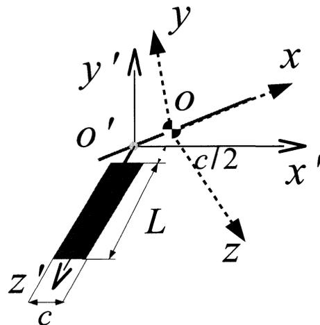
Fig. 3: Two sets of axes fixed to the body ( $o-xyz$ ) and the left forewing ( $o-x'y'z'$ ).
