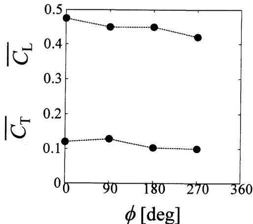
Fig. 10: The time averaged lift coefficient  $\overline{C_L}$  (red) and thrust coefficient  $\overline{C_T}$  (blue) for the 3D flapping wings.
