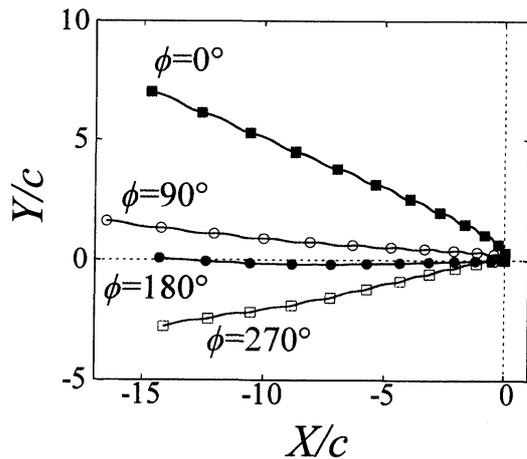
Fig. 9: The trajectories of the center of the mass (COM) for  $0 \leq t \leq 15T$  for the 3D flapping wings. The initial position of the COM is  $(X/c, Y/c) = (0, 0)$ , and the dots indicate the position of the COM when the hindwings are at top dead point.
