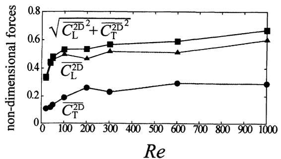
Fig. 6: The time averaged lift coefficient  $\overline{C_L^{2D}}$  (red), thrust coefficient  $\overline{C_T^{2D}}$  (blue), and  $\sqrt{\overline{C_L^{2D}^2} + \overline{C_T^{2D}^2}}$  (black) for  $Re = 20 - 1000$  for the 2D flapping wings.
