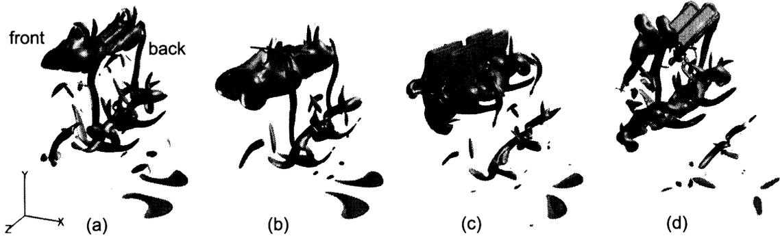
Fig. 7: Isosurfaces of the magnitude of the vorticity ( $|\nabla \times \mathbf{u}|c/u_{\max} = 1.5$ ) around the 3D flapping wings at  $\phi = 0^\circ$ ; (a)  $t = 5.25T$ , (b)  $t = 5.50T$ , (c)  $t = 5.75T$ , and (d)  $t = 6.00T$ .
