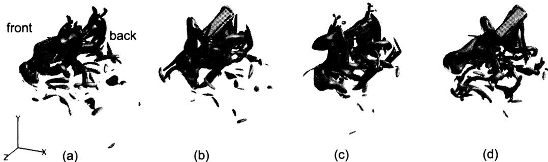
Fig. 8: Isosurfaces of the magnitude of the vorticity ( $|\nabla \times \mathbf{u}|c/u_{\max} = 1.5$ ) around the 3D flapping wings at  $\phi = 180^\circ$ ; (a)  $t = 5.25T$ , (b)  $t = 5.50T$ , (c)  $t = 5.75T$ , and (d)  $t = 6.00T$ .
