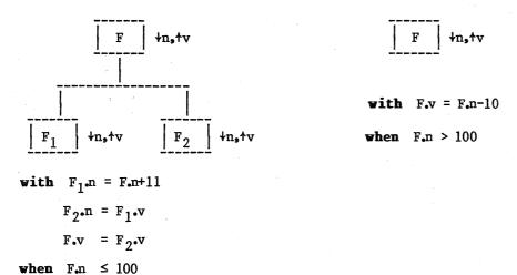
In decomposition 1, module name F is indexed to distinguish different occurrences and no submodule exists in decomposition 2 to terminate decomposition. Attributes prefixed by '\' and '\' are inputs and outputs respectively. The when clause specifies the condition on which the decomposition may apply.
