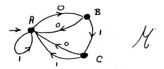
tells us that if we are given the instructions 1010 we are to leave from the initial state A, then 1 sends us back onto A, 0 onto B, 1 onto C, 0 onto A. Any finite string of 0's 1's will send us onto one of the final states A,B or C.
