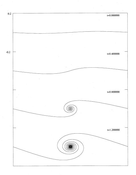
Figure 1: Time evolution of the vortex sheet. G = 0. Krasny's result is reproduced accurately. The scales of the x- and y- axes are slightly different, which make our rolls look more oblate than Krasny's. But this is simply a matter of scaling, only.
