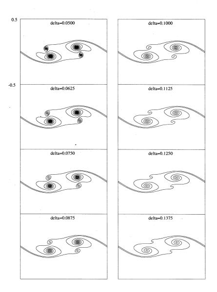
Figure 8: The core region of vortex sheet with various  $\delta$ . The core structure looks universal except for rotating number of roll-ups.
