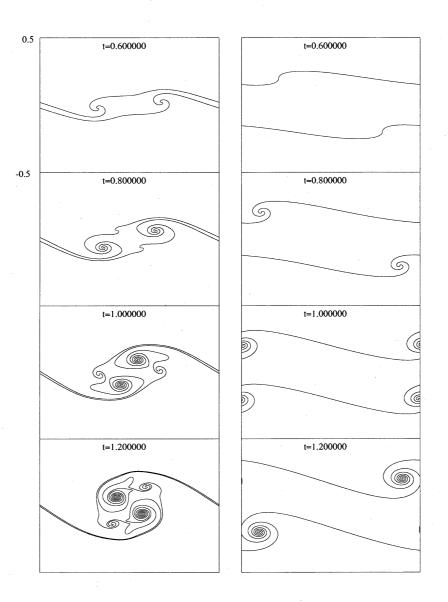
Figure 9: The time evolution of two vortex sheets with the same vorticity. The initial distance between sheets H = 0.4 in the right column, and H = 0.08 in the left column. Their initial phase difference are  $\alpha = 0$ .
