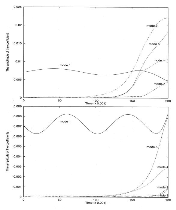
Figure 6: Time evolution of the Fourier coefficients  $a_n = 1 \cdots G = 1.5\pi$  (Upper),  $G = 2.5\pi$  (Lower).
