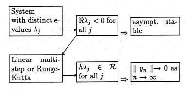
Figure 1.3: Syntax diagram of absolute stability
