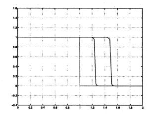
(M = 0.04 and M = 1.0). We can see that overturning will develop if M is not large enough, and if it is sufficiently large, this coefficient does not affect the shock speed as predicted in [9]. We also compute the approximation obtained with no diffusion term (i.e. M = 0) and plot it (green curve) against the one obtained from M = 0.2 (blue curve), and show that the "equal-area" entropy condition is satisfied by the latter (blue curve). See figure 8.
