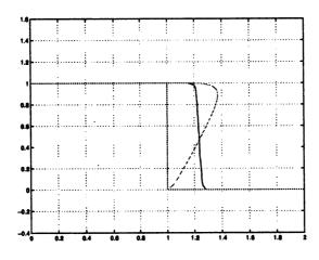
Figure 9: Numerical solution (WENO5-LLF) to the Burgers Equation with sine wave as initial data. We plotted the zero level set at time t = 0 and 0.5.
