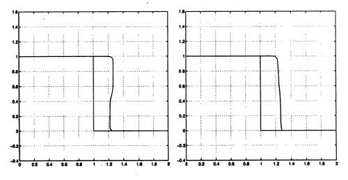
Figure 8: Numerical solution to the Riemann problem of Burgers' Equation with  $u_L = 1.0$ ,  $u_R = 0.0$ . We plotted the zero level sets at time t = 0 and 0.5 obtained from M = 0.2 and 0.0.
