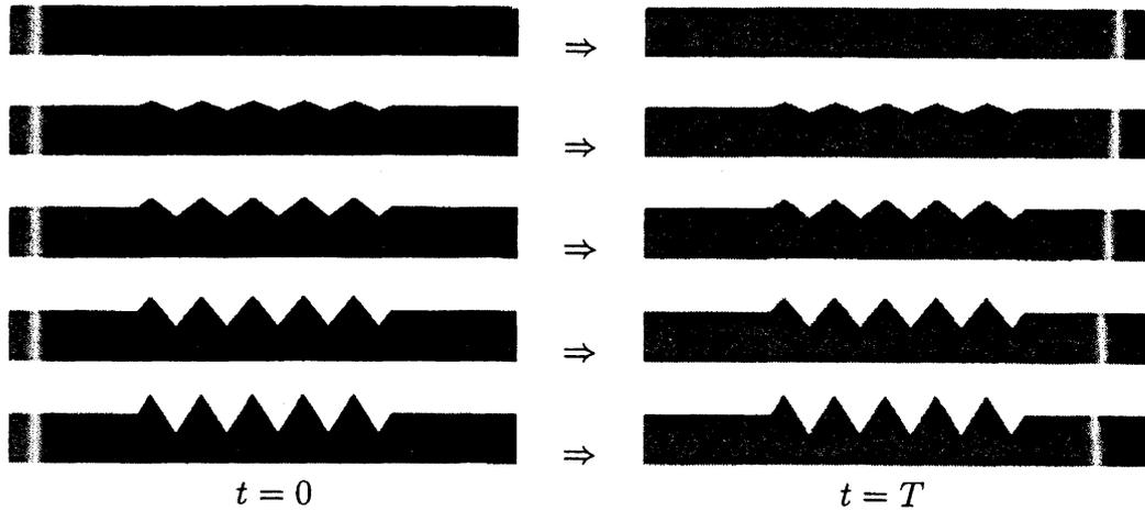
FIGURE 1. Numerical simulations of front propagation for (1.2) in five different domains when  $\varepsilon = 0.050$ ,  $f(u) = u(1 - u)(u - 1/4)$ . The white region approximately represents the position of the front.
