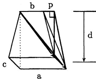
$$V = \frac{1}{3}acd + \frac{1}{3} \times \frac{1}{2}cd(b + P) - \frac{1}{3} \times \frac{1}{2}cdP = \frac{2acd + bcd}{6}$$
