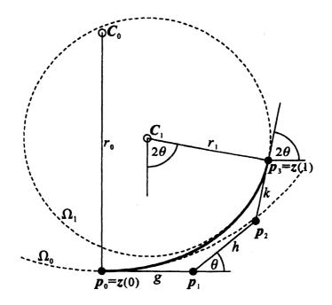
Figure 1: Circle to circle transition with single cubic spiral.
