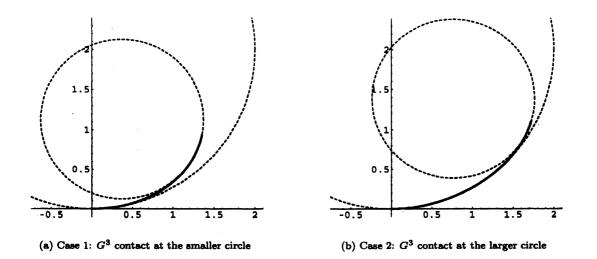
Figure 4:  $G^2$  cubic Bézier spiral transition between two circles.
