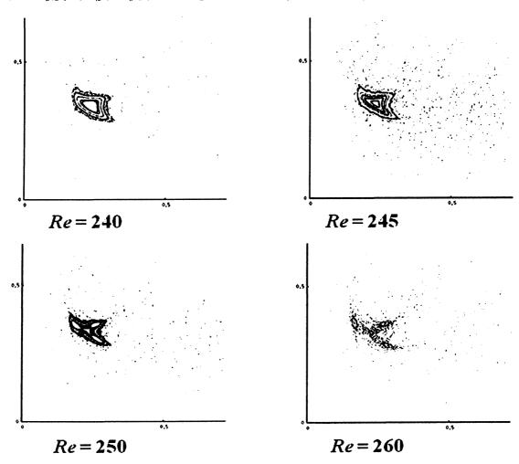
☑ 3 Poincaré sections near the 3:1 resonance
