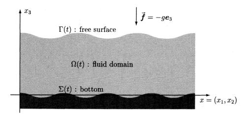
The functions b and  $\eta$  represent the bottom topography and the surface elevation, respectively. It is very important to predict the deformation process of the seabed, so that we have to analyze the behavior of this function b. However, in this communication we assume that b is a given function and we concentrate our attention on analyzing the behavior of the function  $\eta$ , namely, the water surface.
