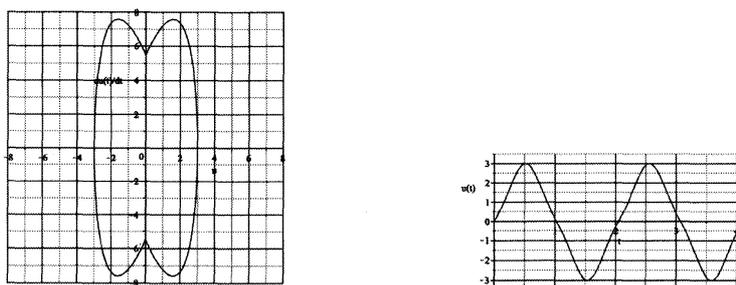
Figure 4.4: (left):The “single-time oscillation” orbit with the initial condition:  $u(0) = 0, \dot{u}(0) = \sqrt{30}$  in Example 4.1.  $\omega \doteq 2.047$ . (right): The time history of the “single-time oscillation” orbit. The time is shown up to two periods.
