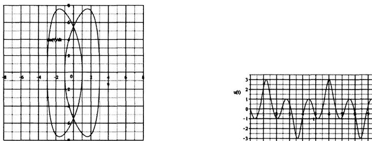
Figure 4.2: (left):The “triple-time oscillations” orbit with the initial condition:  $u(0) = 0, \dot{u}(0) = -\sqrt{30}$  in Example 4.1.  $\omega \doteq 4.808$ . (right): The time history of the “triple-time oscillations” orbit. The time is shown up to two periods.
