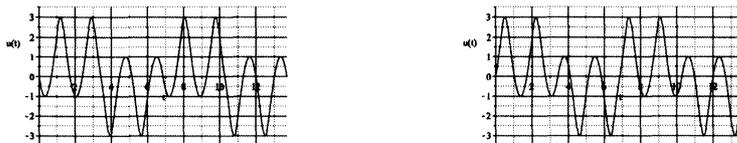
Figure 4.7: (left):The time history of the “quadruple-time oscillations” orbit with the initial condition:  $u(0) = 0, \dot{u}(0) = -\sqrt{30}$ . The time is shown up to two periods.  $\omega \cong 6.856$ . (right): The time history of the “quadruple-time oscillations” orbit with the initial condition:  $u(0) = 0, \dot{u}(0) = \sqrt{30}$ . The time is also shown up to two periods. The orbits of both figures are the same of Figure 4.2 and/or 4.3.
