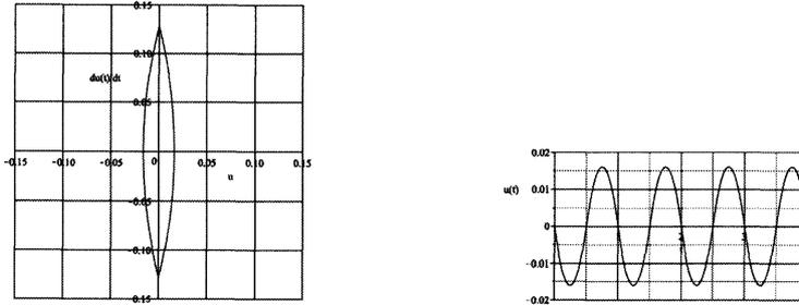
Figure 3.3: (left):The  $\omega(=1)$ -periodic orbit with the initial condition:  $u(0) = 0, \dot{u}(0) = \frac{\cos \frac{1}{2} - 1}{2 \sin \frac{1}{2}} = -0.1276709606\dots$  in Example 3.2. (right):The time histories shown up to four periods.
