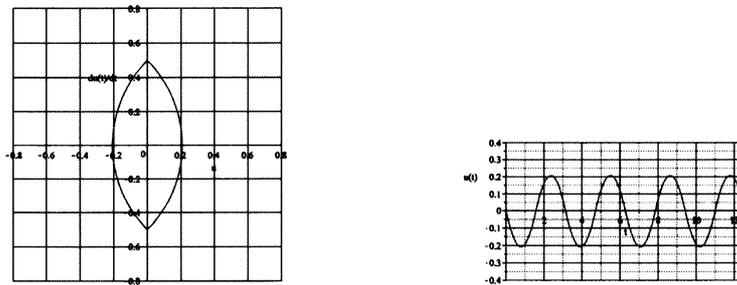
Figure 3.1: (left):The phase portrait of the  $\omega(=\pi)$ -periodic solution in the initial condition:  $u(0) = 0, \dot{u}(0) = -\frac{1}{2}$  in Example 3.1. (right): The time history of the  $\omega(=\pi)$ -periodic solution. The time is shown up to four periods.
