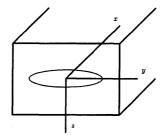
The elliptical shape in the figure above shows the tail, x-axis extends forward in the flow direction, y-axis is along the span of the aerofoil and z-axis indicates the downwash direction.
