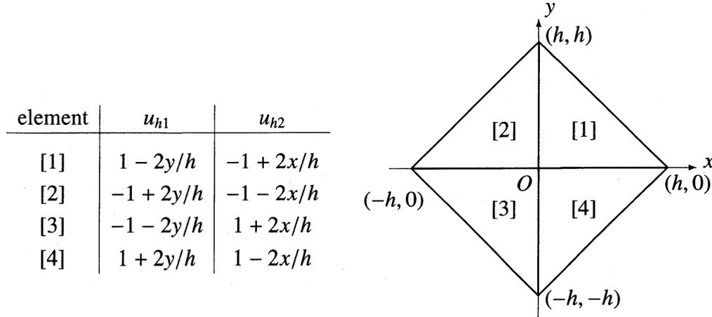
Figure 4: Example of patch of triangular elements
