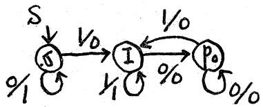
$$\left\{ \begin{array}{l} S \xrightarrow{\sigma} \sigma \\ \sigma \xrightarrow{\sigma} I, \quad \sigma \xrightarrow{0} \sigma \\ I \xrightarrow{1} I, \quad I \xrightarrow{0} P_0 \\ P_0 \xrightarrow{1} I, \quad P_0 \xrightarrow{0} P_0 \end{array} \right.$$
