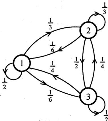
Fig. 1. The state diagram for the Markov source.
