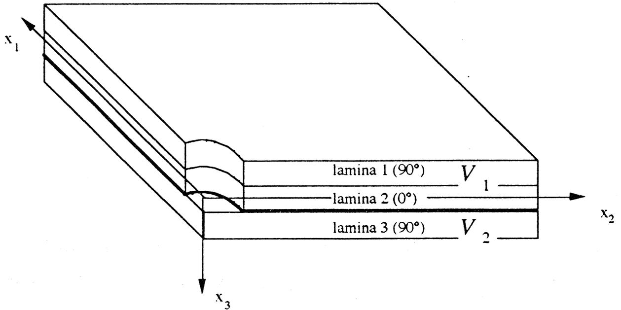
Figure 1 - A quarter of a cross-ply laminate with a hole in the first two laminae
