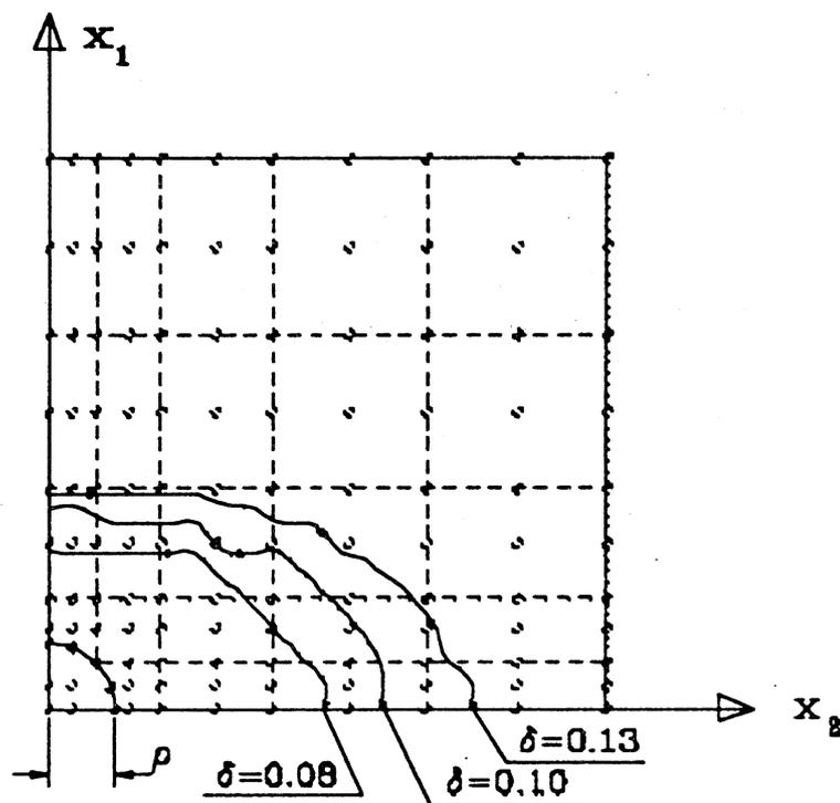
Figure 2 - Zones in adhesion and delaminated for  $\delta = 0.08, 0.10$  and  $0.13$  cm
