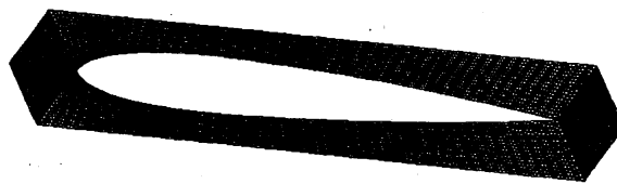
Fig. 3: Triangular element (8,192 elements)
