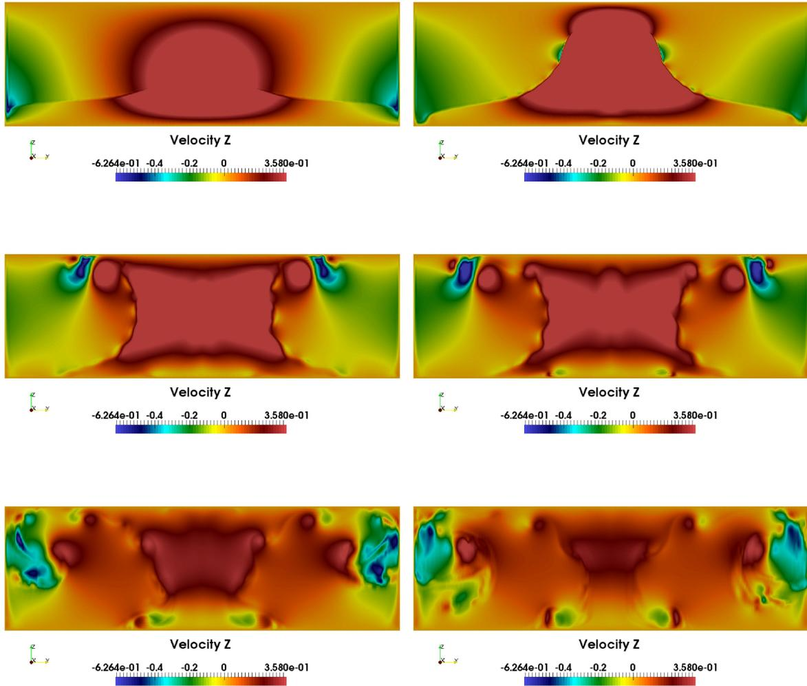
Figure 1: Time evolution of the axial velocity  $u_z$  on the plane  $x_1 = 0$  in the no swirl case with  $Re = 50,000$ .  $t = 0.1$  (top left),  $0.3$  (top right),  $1.0$  (middle left),  $1.3$  (middle right),  $2.3$  (bottom left) and  $3.0$  (bottom right). Note that the red and blue colors represent positive and negative values in this figure.
