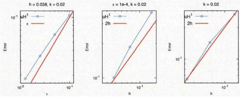
Figure 2: (left) The error  $\|u_f^M - u_h^M\|_{H^1(\Omega)}$  for different penalty parameter  $\epsilon$  with fixed mesh size  $h = 0.038$  and  $\Delta t = 0.02$ . (middle) The error  $\|u_f^M - u_h^M\|_{H^1(\Omega)}$  for different mesh size  $h$  with fixed penalty parameter  $\epsilon = 10^{-4}$  and  $\Delta t = 0.02$ . (right) The error  $\|u_f^M - u_h^M\|_{H^1(\Omega)}$  for different mesh size  $h$  with  $\Delta t = 0.02$  for the Lagrange multiplier approach.
