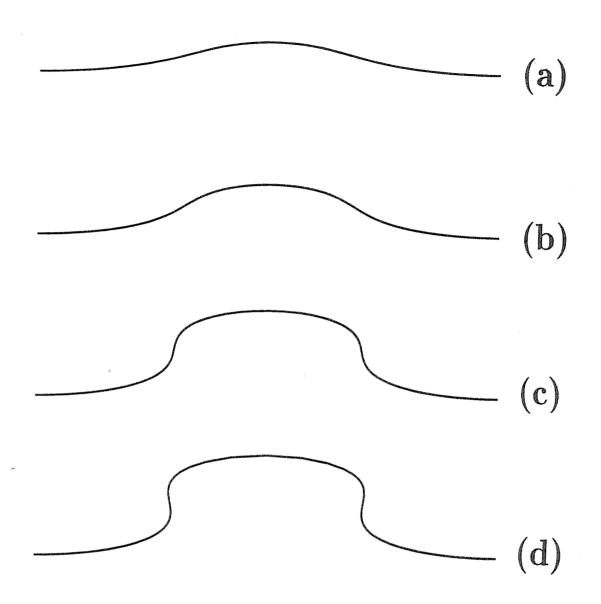
Figure 2: Wave profiles for  $q=-0.5(a),\ -1.0(b),\ -2.25(c),\ -3.0(d).$  N is equal to 255, 511, 1023, 1023, respectively.
