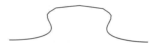
Figure 3: Wave profile for q=-4.0. The truncation is N=1023. Insufficiency of the modes are clearly seen at the crest.
